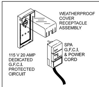
The Ground Fault Circuit Interrupter (GFCI) is located at the end of the power cord. This device is for your protection. It is very important to protect it from rain and other moisture. Test once a month, with the plug connected to the power supply,
